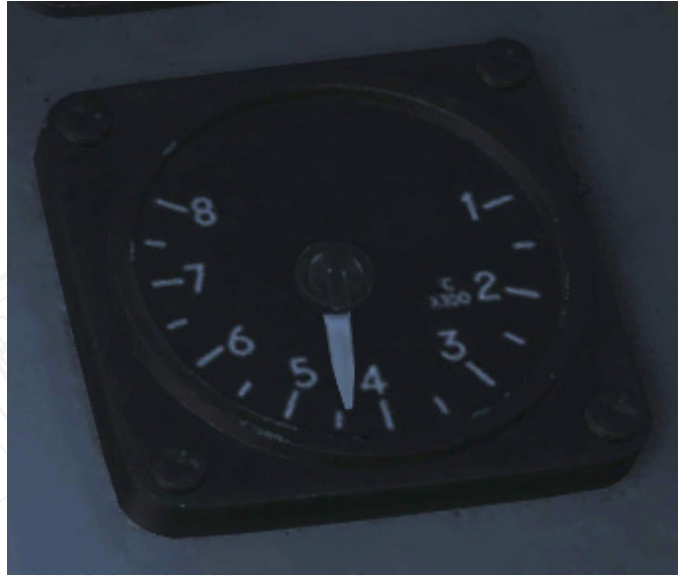
Figure 16 EGT indicator. Approximately. 440°
