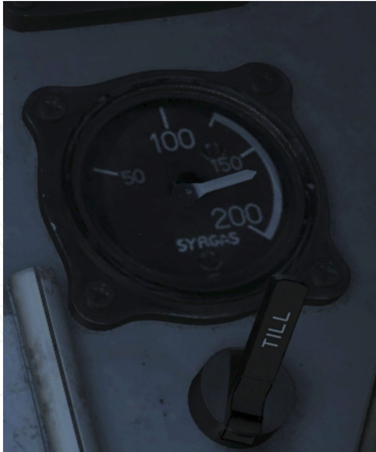
Figure 168 Oxygen pressure indicator (kp/cm 2 ) and oxygen valve ON (TILL)
