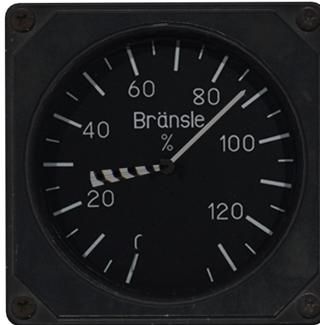
Figure 129 Fuel indicator. 87% fuel remaining. Striped “tie” indicating approx. 30% required to complete flight plan with fuel reserve included.
