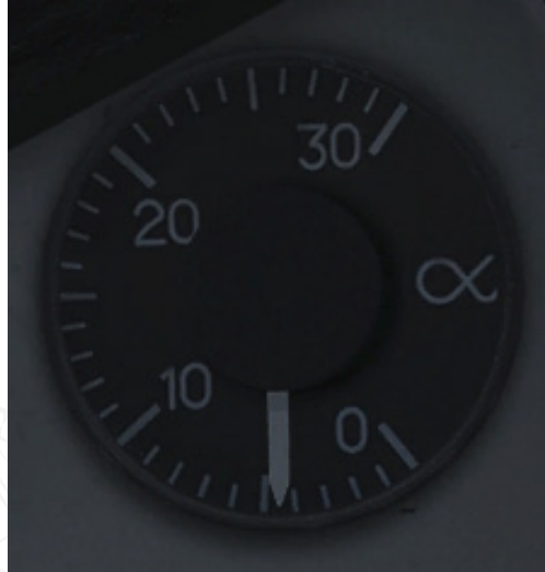
Figure 12. Angle of attack indicator. Indicating 4.5° AoA ( \alpha ).
