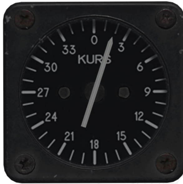
Figure 21. Backup Compass. Indicating 020° Magnetic.
