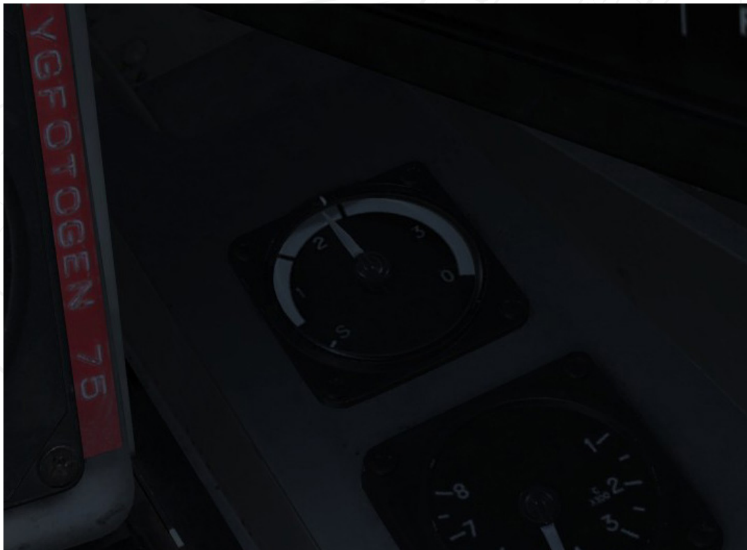
Figure 45 Engine nozzle indicator. Zone 2 afterburner open.
