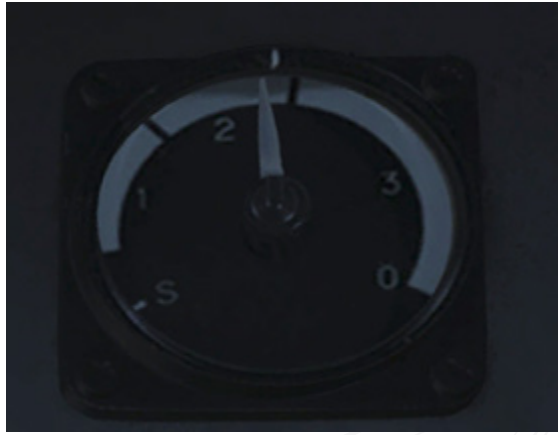
Figure 18. Engine nozzle indicator. Zone 2 afterburner open.
