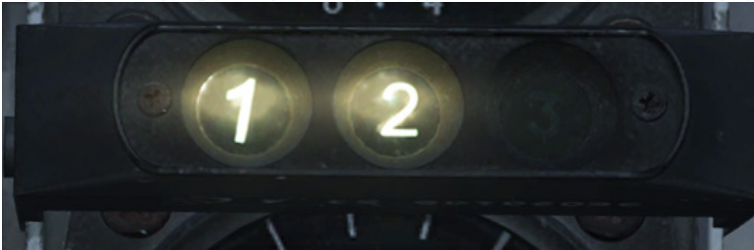
Figure 17. Afterburner indicator. Afterburner Zone 2 selected.
