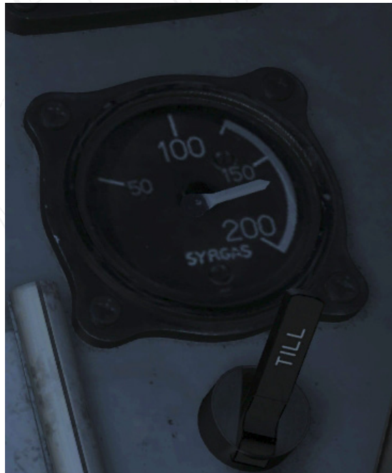
Figure 28 Oxygen pressure indicator. >150 kp/cm 2 remaining. Oxygen valve in the ON (TILL) position.
