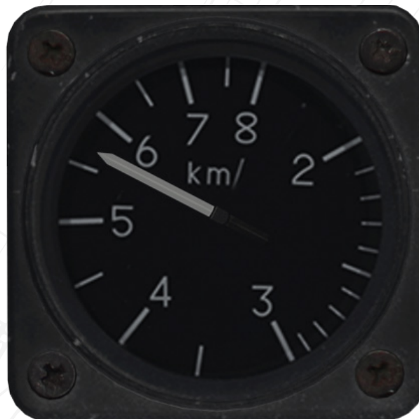
Figure 22 Backup airspeed indicator. 560 km/h indicated airspeed.
