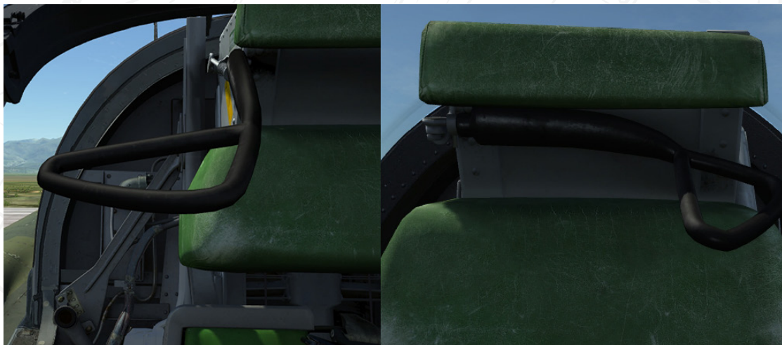
Figure 167 Ejection seat arming lever. Left SAFE, Right (stowed) UNSAFE.
