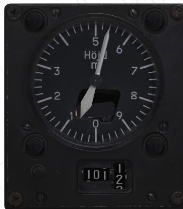
Figure 10. Main altimeter. 520 m altitude. Pressure set to 1011.5 hPa.
