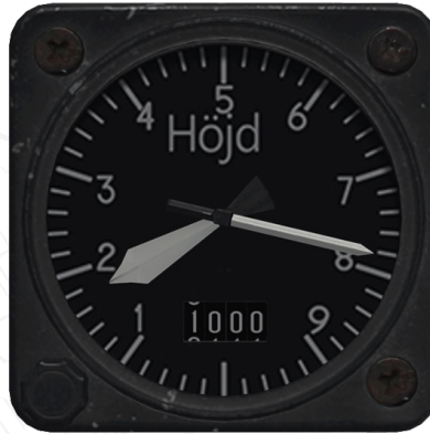
Figure 19 Backup Altimeter. 1780 metres. Pressure set to 1000 hPa.
