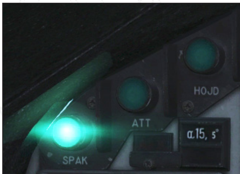
Figure 62 Autopilot mode selector buttons. SPAK mode on.
