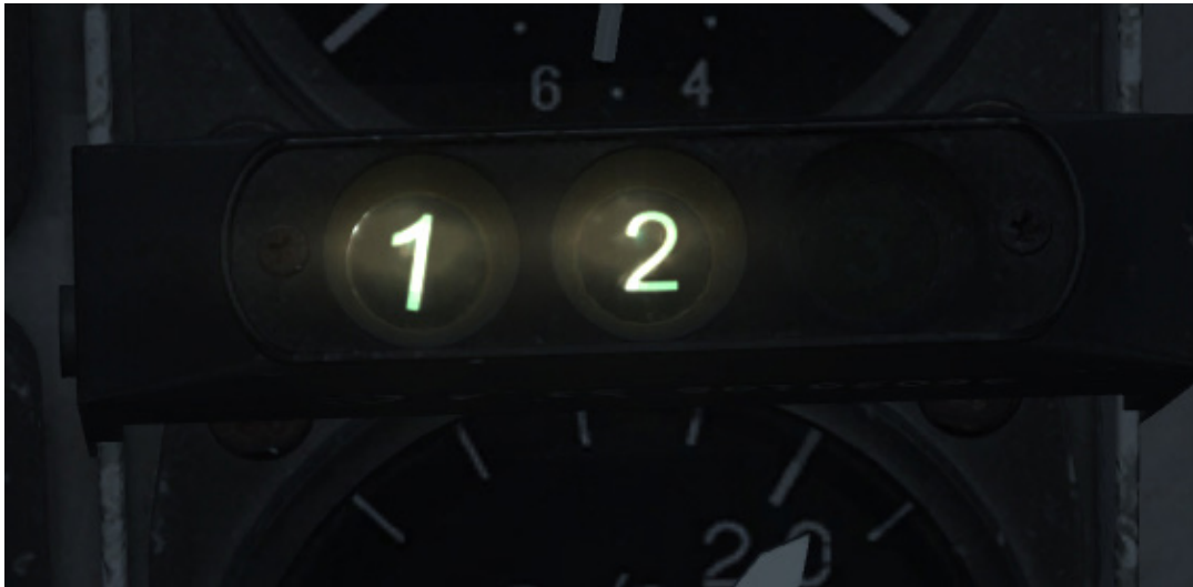
Figure 44 Afterburner zone indicator. Zone 2 selected.
