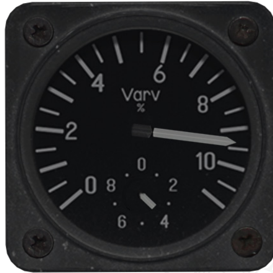
Figure 14. RPM indicator. 94% RPM.
