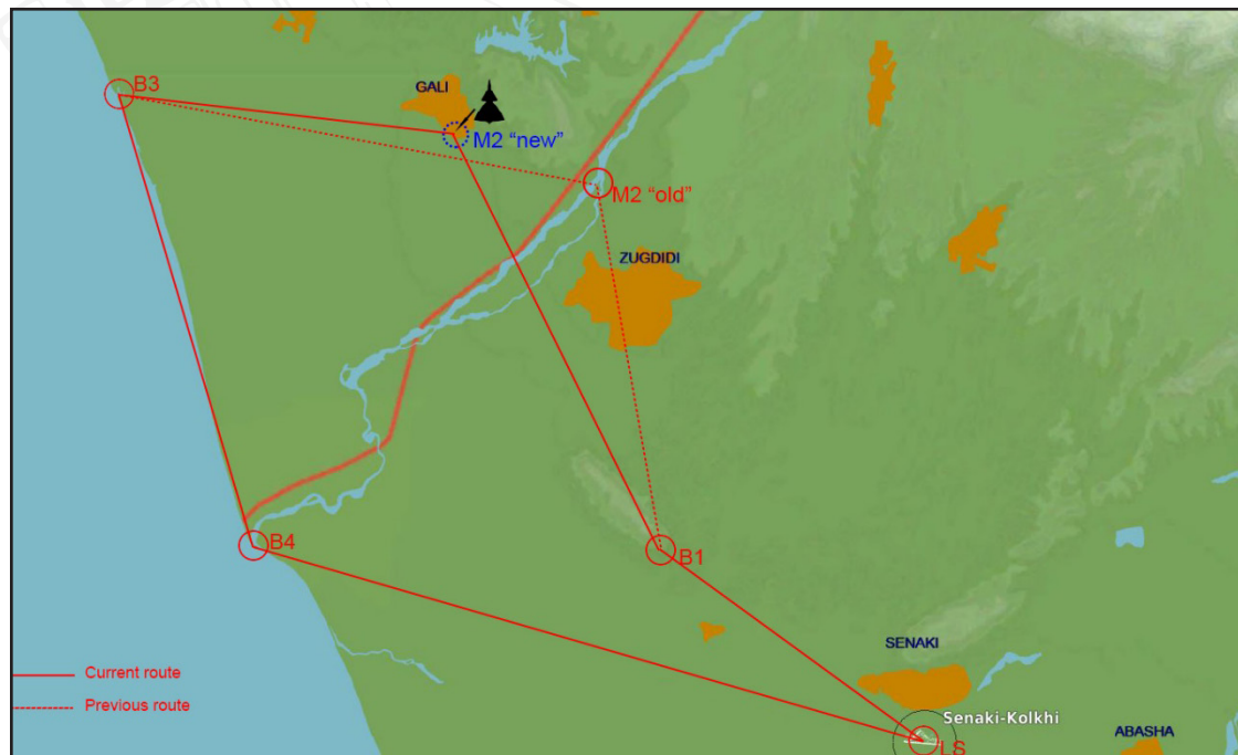
Figure 121 In this case, the target position M2 is moved via a visual target fix (or weapons impact fix) from the island in the river “M2 old” to the outskirts of Gali “M2 new”. Only the current selected target waypoint is moved and the rest of the navigation polygon is unaffected.
